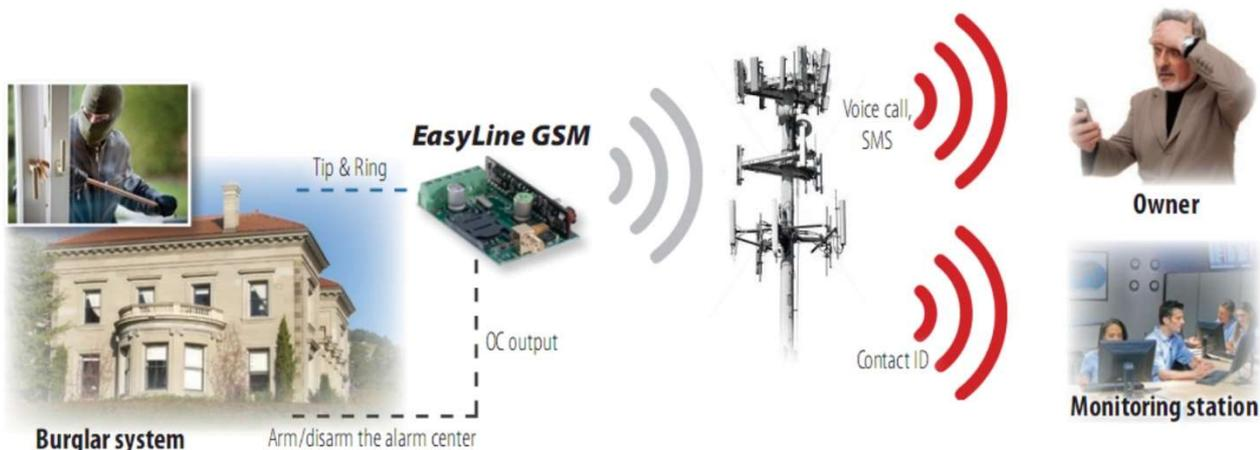
**Figure 1: Device operation**
